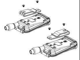
The Belt Clip can be reversed to change the access direction of the stereo jack.
